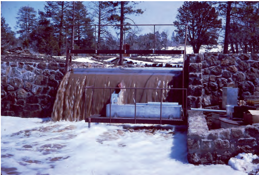
Figure 6.3. A series of splitters established to sample suspended sediment in the streamflow passing through the spillway of a dam (photograph by Peter F. Ffolliott).
