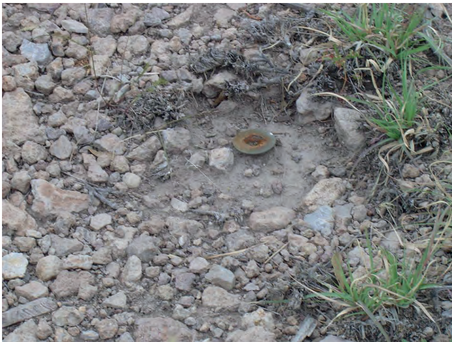
Figure 2.2. An erosion pin consisting of metal nail with a washer welded to the top of the nail inserted into the soil surface to measure surface erosion. The distance between the cap of the pin and the soil surface is a measure of surface erosion (photograph by Peter F. Ffolliott).
