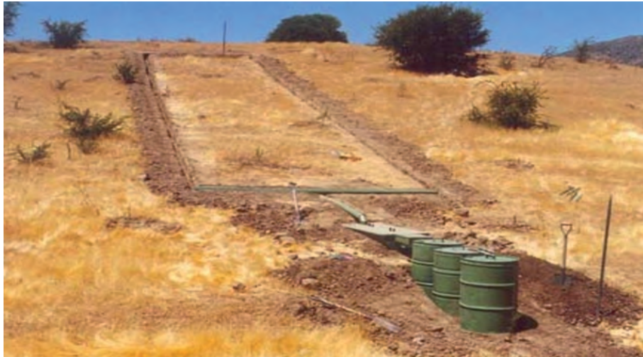
Figure 2.1. A bounded plot for quantifying surface erosion by measuring the amount of soil that washes from the plot (photograph by Roberto Pizarro Tapia).
